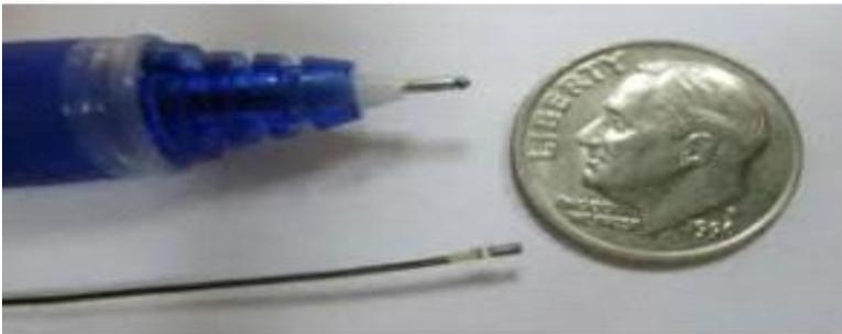
Good thing Medigus made the world's smallest video camera so those medical probes are a little less painful. It's .99mm in diameter... iApp Endoscope for iPhone5s packs 7 Endoscopes via wifi in different hidden locations and more... via iApps!!
